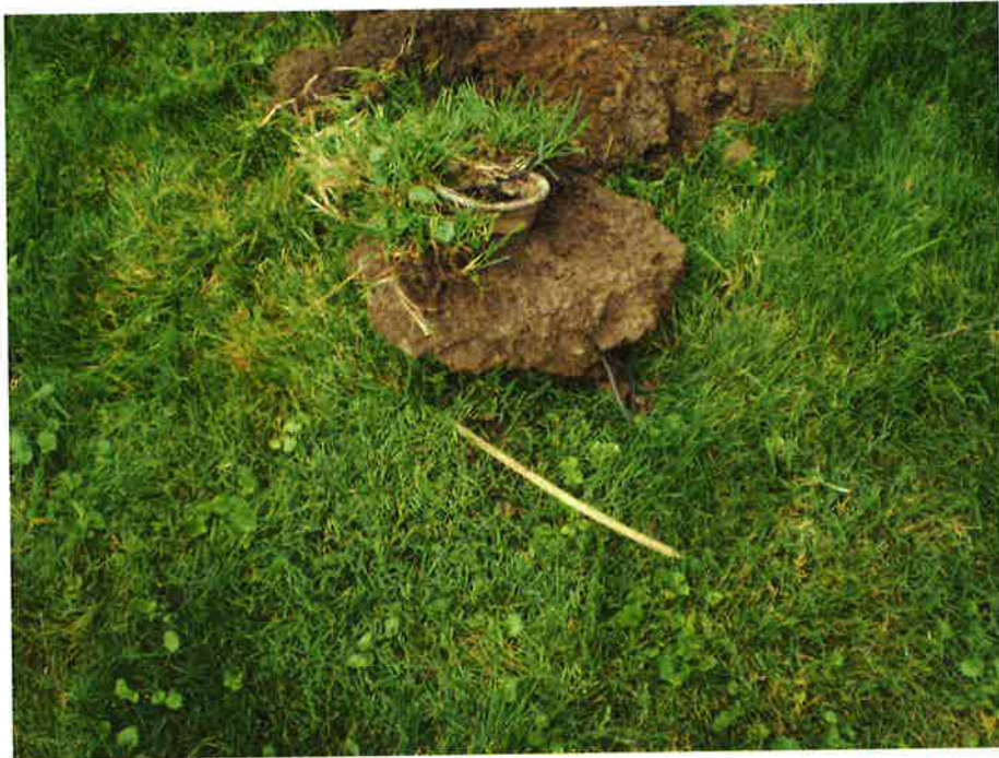
Photo 7. MP-7T(?) flush mount protective casing and tubing that had been installed in this probe location.
