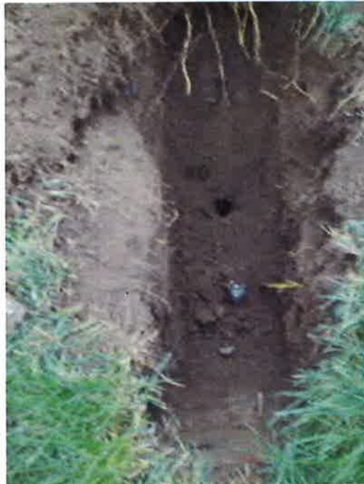
Photo 5. Excavation for SP-2 and SP-2R. One casing has been partially pulled up during excavation.
