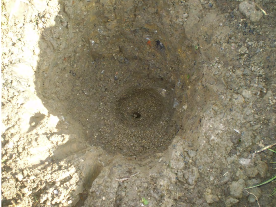
Photo 5. MP-10 excavated to 3 feet with screen removed.
