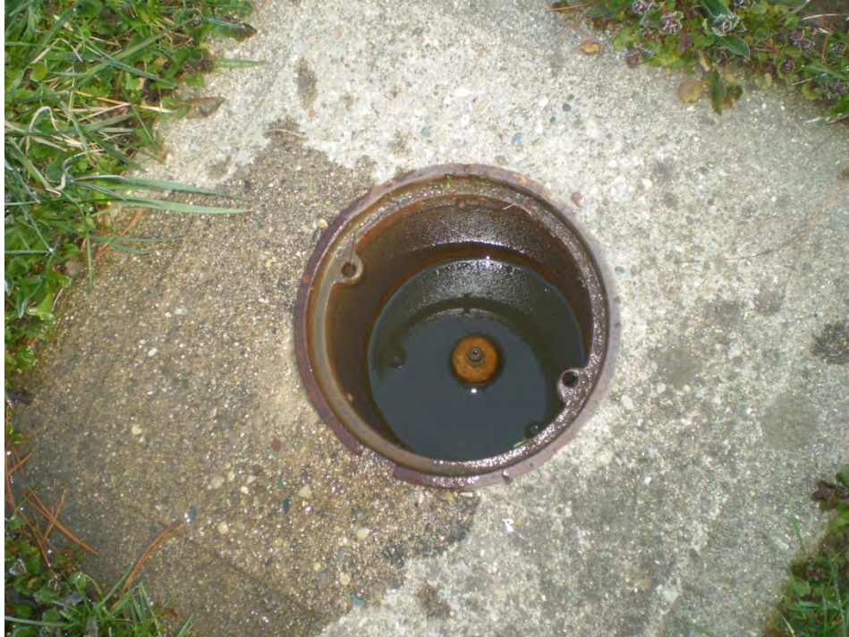
Photo 3. MP-10 bailed to expose cap and quick connect.
